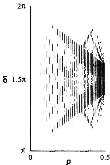
Fig. 5. The location of the barriers in the wavelength for the transmission coefficients for  $n_A/n_B = 2.0$ . The vertical line indicates  $\delta$  between  $\pi$  and  $2\pi$ , while the horizontal line indicates the density of B to A layers.
