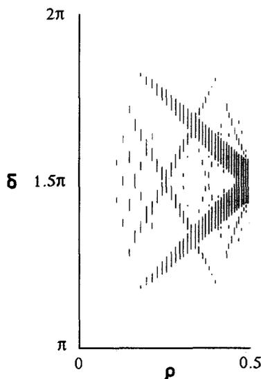
Fig. 4. The location of the barriers in the wavelength for the transmission coefficients for  $n_A/n_B = 1.5$ . The vertical line indicates  $\delta$  between  $\pi$  and  $2\pi$ , while the horizontal line indicates the density of B to A layers.
