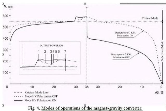
Fig. 4. Modes of operations of the magnet-gravity converter.
